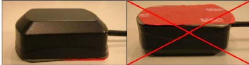
Figure 27 GPS antenna correct mounting.
